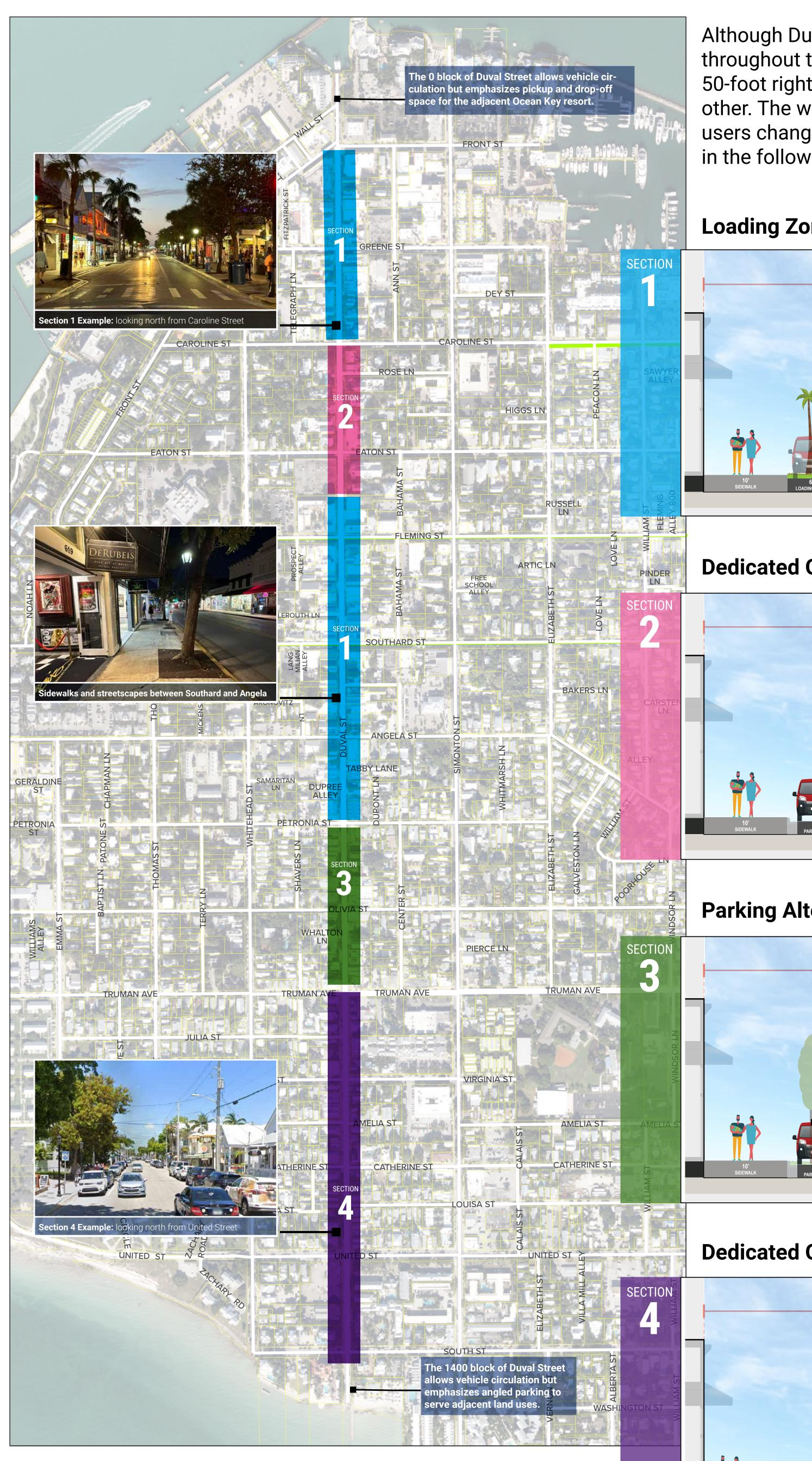
Although Duval Street's travel patterns change throughout the corridor, the street has a constant 50-foot right-of-way width from one end to the other. The way this 50 feet is allocated to different users changes throughout the corridor, as shown in the following section illustrations.
